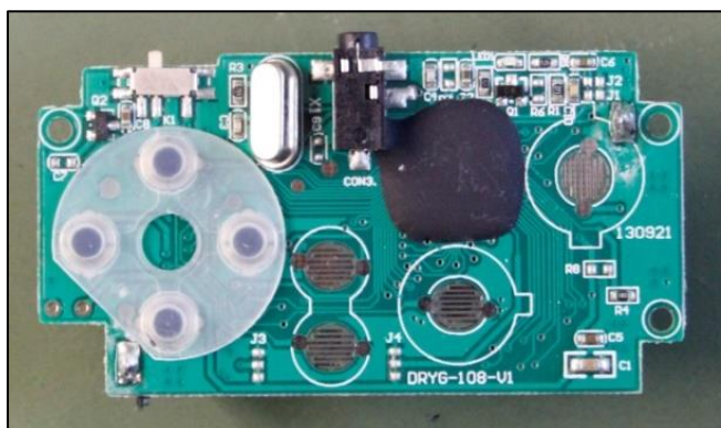
Upper side with quartz, connector and controller
